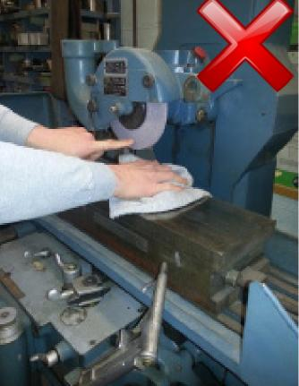
Do not pass hand under rotating grinding wheel.
