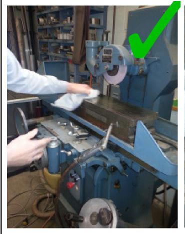
Move table/wheel out of the way to clear hand while cleaning chuck.
