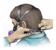
4. Adjust all the straps equally on both sides of the respirator.
