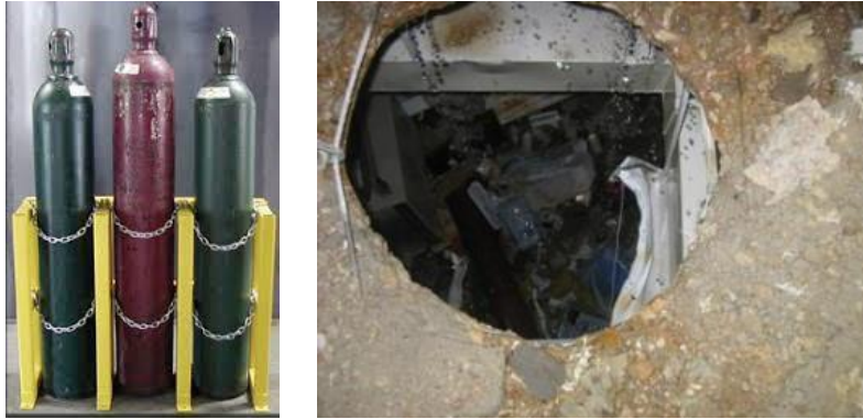
Figure 6-7: Correct way to storage compressed gas cylinders (left). Damage caused by a compressed gas cylinder (right).
