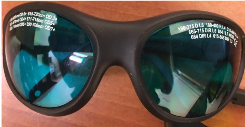
Figure 7-27: Laser goggles labels. In the left filter are the labels complying with the ANSI standard. On the right filter are the labels complying with the international standard.
