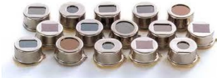
Figure 8-17: Pyroelectric effect (left). Pyroelectric detectors (right).
