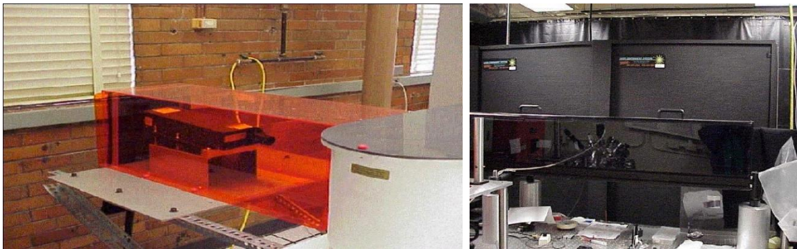
Figure 7-10: Plastic beam enclosure that is transparent to many wavelengths but absorbs the laser wavelength (left). Metallic beam enclosure which is completely opaque (right).
