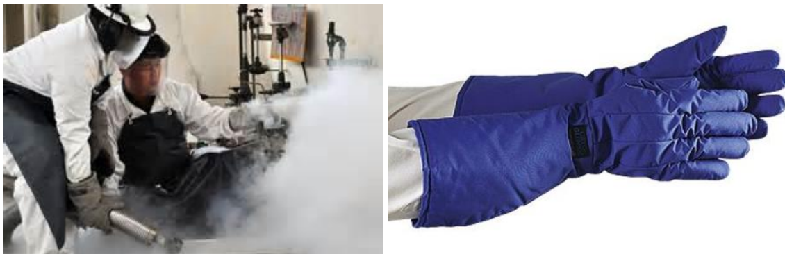
Figure 6-5: Cryogenic hazards (left). Gloves used when handling cryogenic liquids (right).
