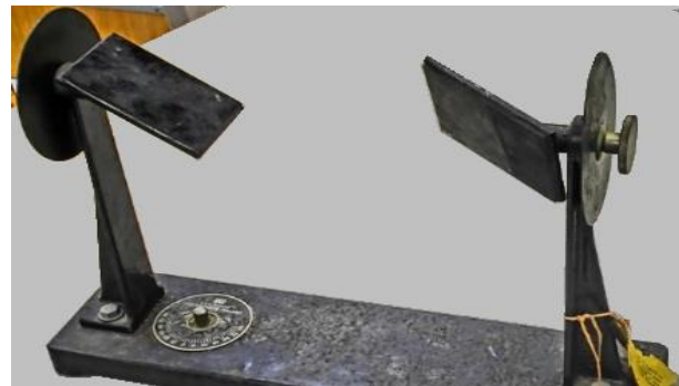
Figure 2-37 : Reflection and refraction of an unpolarized beam hitting the interface at Brewster's angle (left). : Two mirrors mounted at Brewster's angle (right).
