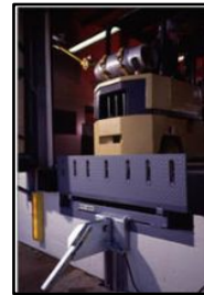
Dock Leveler and Barrier
