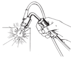
Figure 41-9: Fume Extraction Gun
