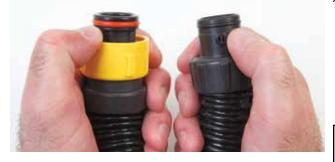
When using the PA031 and PA031L, verify that the o-rings are installed on both end connectors. When using the PA034 or PA034L, verify that the o-ring is installed on the blower-side connector. Inspect the o-rings for any damage. If an o-ring is missing or damaged, do not use the breathing tube. Replace the missing or damaged o-ring.
